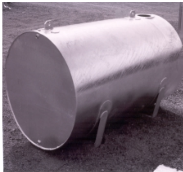
Large tanks require large drain holes. This tank will contain over 7 tonnes of molten zinc when immersed, which must be able to flow in and out freely.
